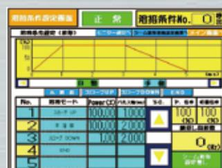
溶接条件設定画面／Welding condition setting screen
